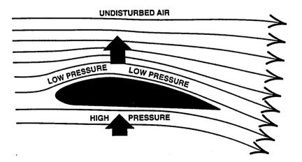
Wings on aircraft are cambered (arched) on top to create LIFT. How? The curved shape forces the air flowing over the wing to move faster than the air flowing under the wing. According to Bernoulli's Principle (see the Aviator's Glossary), this faster-moving stream of air has lower air pressure relative to the pressure below the wing. The higher pressure area below forces the wing upward. That's LIFT!
